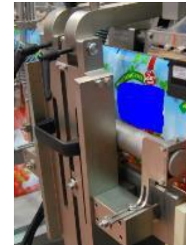
BOTTOM SEAL COOLING WHEN MACHINE STOPS; AIR BLOWN TOWARDS THE BOTTOM SEAL WHEN MACHINE STOPS Requires software modifications.
